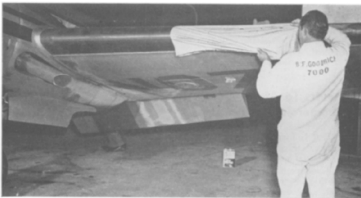
FILM STRIPPING —A thin film is applied on airplane de-icers to protect the rubber from hot weather. At the end of the season it can be stripped off as shown.
